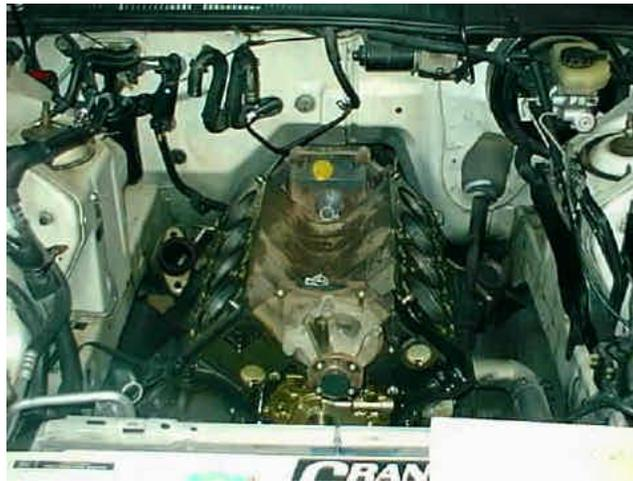
Here is a picture of my engine with the heads removed.
