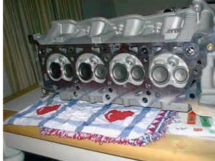
You can see the shape of the intake ports is more square, versus the tear shape on the old heads.
